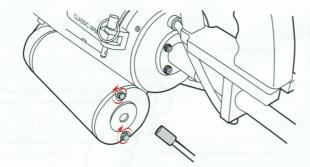
Remove the cover and pull out the connector.
