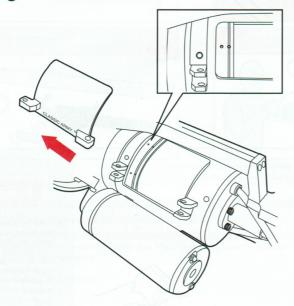
After adjustment turn the barrel to check if the dial is too loose.
