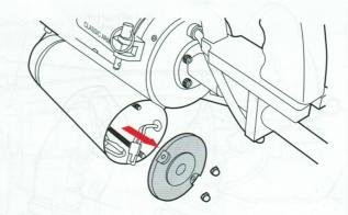
3 Connect the battery to the connector.
