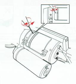
Put the cover back on and lock it with the two pins.
