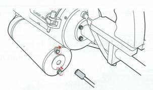
6 Press the trigger to test the rotation of the barrel. It should turn anti-clocwise.
